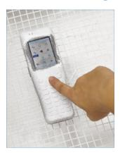
The DT-X8 is shock protected against drops from height of up to 3 metres onto concrete. This completely covers all impacts and fall heights that typically occur in a warehouse. The terminal withstands dust and temporary immersion in water in accordance with protection class IP67 and it works at temperatures down to -20°C. This guarantees that the device can be used outdoors the whole year, as well as in cold stores, wet areas and in particularly dusty or dirty environments.
